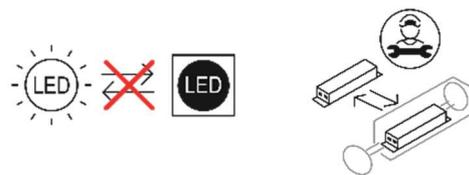
\*Do not connect the luminaire to an active LED driver. Some LED drivers emit high voltage when idle, which may cause permanent damage to the luminaire. Be sure to disconnect the LED driver from the power line before connecting the luminaire.
