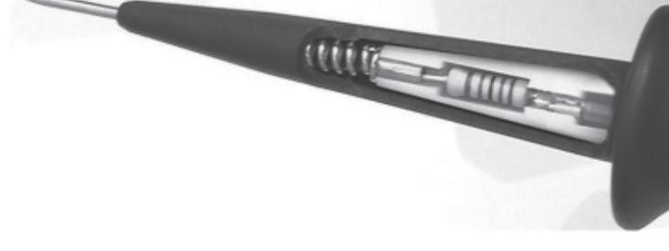
The instrument provides a high level of safety by means of two series resistors immediately behind the test electrodes as well as two absolutely independently working test systems.
