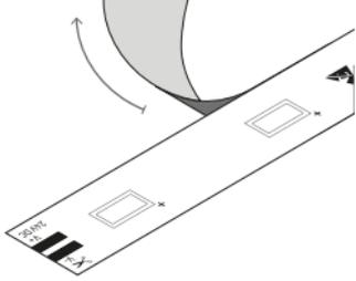
**Never fasten the LED strip over a profile joint!** The physical expansion or contraction of the profile in the event of temperature fluctuations may damage the LED strip. A solution here is to cut the solder pads at the profile joint and to use flexible connections, e.g. soldered flexible wire bridges or LED strip connectors.
